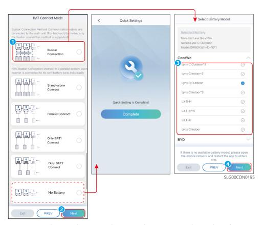
**Step 8**Set the working mode according to actual needs. After setting, please click. **Next step**, Work mode configuration completed. For certain models, after the work mode configuration is completed, the system automatically enters the CT/meter self-test state. During this process, Inverter will temporarily disconnect from the grid and then automatically reconnect.
