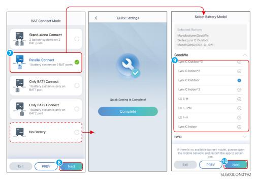
For certain models, when paralleling Inverter via RS485, please set the Battery access mode to either busbar mode or non-busbar mode based on actual conditions, and select the Battery model. Once the master unit is configured, the slave units will automatically synchronize the Battery settings. If the Battery connected to the slave unit does not match the master unit, please access the Quick Settings interface via the slave SN on the homepage and configure the Battery model separately.
