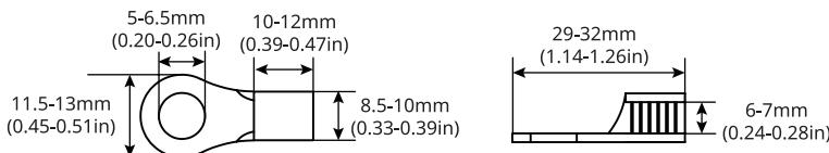
**Step 1:** Strip the insulation layer and insert the bared conductor into the terminal.
