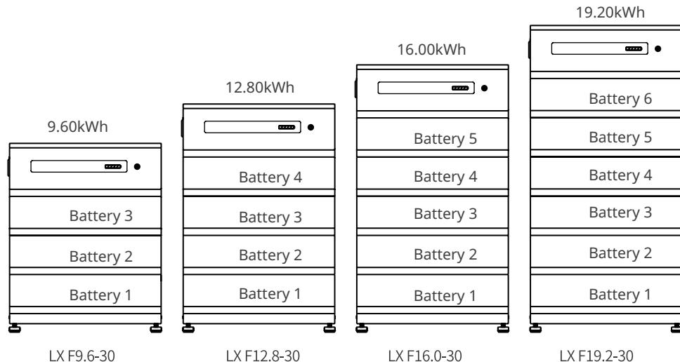
A max of eight battery systems can be parallel connected in one energy storage system. Ensure that the usable energy of each battery system is the same.
