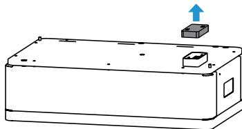
**Step 1:** Install the adjustable feet to the base.
